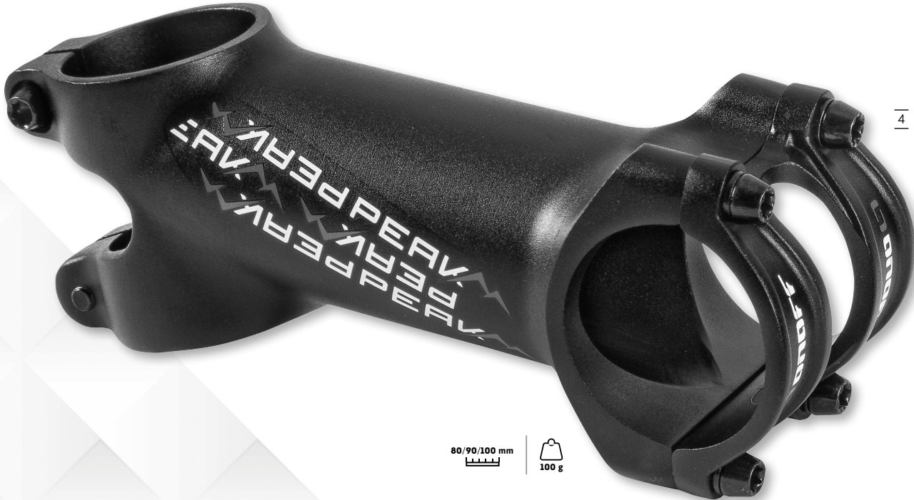
3 PEAK STEM 6° · 3D forged AL7050 · Ultra-light-weight alloy · Bar bore: 31.8mm · Rise: ±6° · Length: 80 / 90 / 100mm · Weight: 90g (90mm length)
