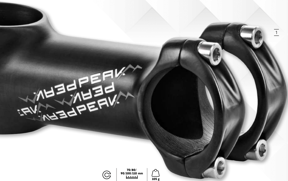
1 PEAK STEM CARBON 6° · UD Carbon + AL7050-T731 · Bar bore: 31.8mm · Rise: ± 6° · Length: 70 / 80 / 90 / 100 / 110mm · Weight: 105g (90mm length)
