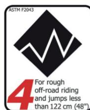
This is a set of conditions for operation of a bicycle/component that includes Conditions 1, 2, and 3, or downhill grades on rough trails at speeds less than 40 km/h (25 mph), or both. Jumps are intended to be less than 122 cm (48 in.).
