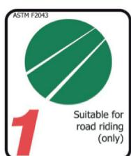
This is a set of conditions for the operation of a bicycle/component on a regular paved surface where the tires are intended to maintain ground contact.
