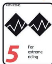
This is a set of conditions for operation of a bicycle/component that includes Conditions 1, 2, 3, and 4; extreme jumping; or downhill grades on rough trails at speeds in excess of 40 km/h (25 mph); or a combination thereof. **Not covered is the area of use dirt bike!**
