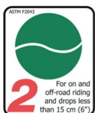
This is a set of conditions for the operation of a bicycle/component that includes Condition 1 as well as unpaved and gravel roads and trails with moderate grades. In this set of conditions, contact with
